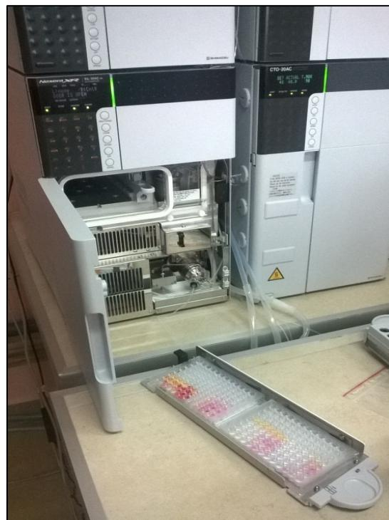
**Fig. 2.** UHPLC Nexera XR Shimadzu. SIL-20ACXR autosampler equipped with MTP holder (Photo: P. Stalica).
