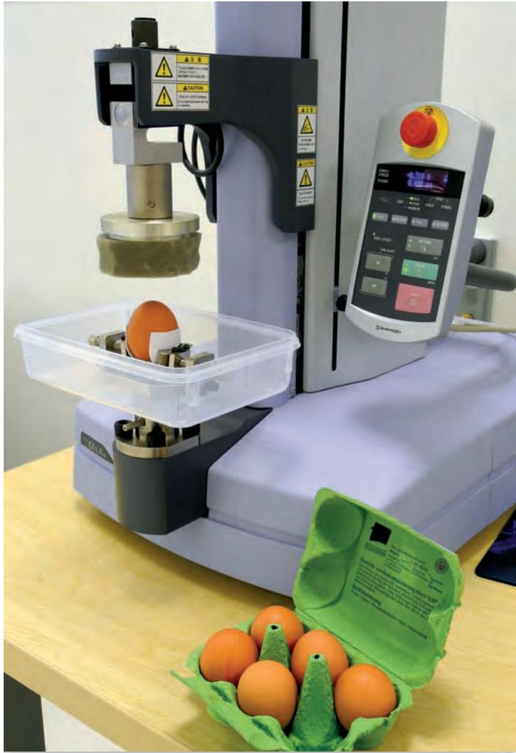
Figure 1: Texture Analyzer EZ-Test-LX with customized compression jig
