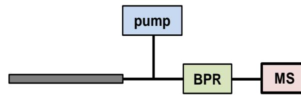
C: Full flow through BPR with make-up pump
