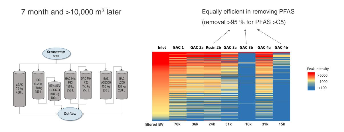
Even though GAC and Resin seem equally good in removing PFAS, differences in overall cleaning efficiency are observed
