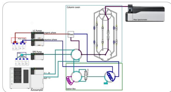
Figure 1. Schema SPE on-line UHPLC-MS/MS (Number of patent : WO 2016/098169 A1).
