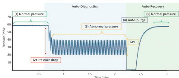
Fig. 7 Diagram of Auto-Diagnostics and Auto-Recovery Functions
