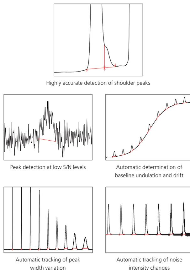
Fig. 8 Example of Automatic Peak Integration Using i-PeakFinder
