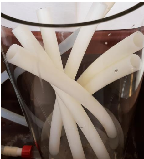
Figure 1 Hoses being rinsed for 60 minutes
