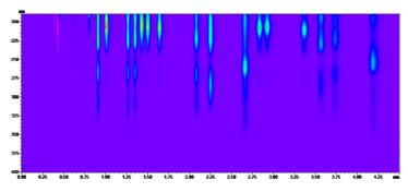
Analysis of 16 Cannabinoids with the Shimadzu Nexera-i (LC-2040C 3D) UHPLC with PDA
