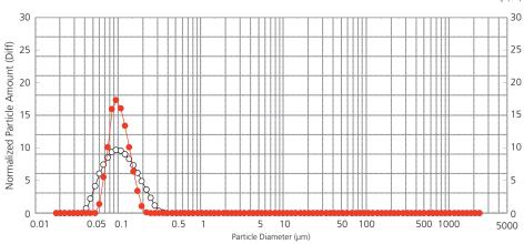
Example of a narrow, nanometer, monomodal distribution of particles
