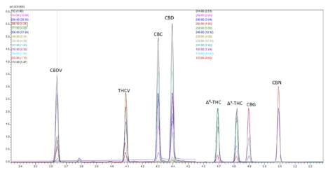
Analysis of 11 Cannabinoids with Shimadzu's GCMS
