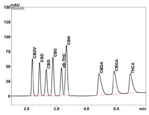
Analysis of 9 cannabinoids with Shimadzu's Nexera UC SFC system
