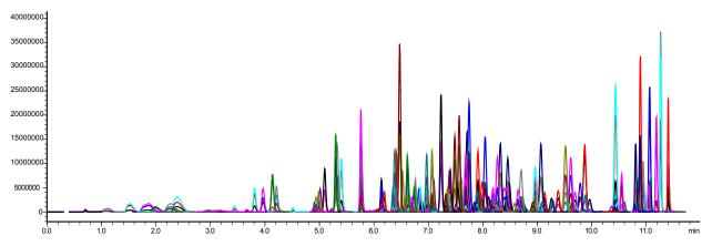
High-sensitivity LC-MS/MS analysis of 211 pesticides in cannabis dry product in less than 12 minutes using a Shimadzu LCMS-8060 triple quadruple mass spectrometer
