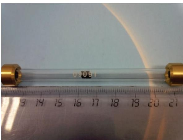
Figure 2: Sample placed into the TD tube
