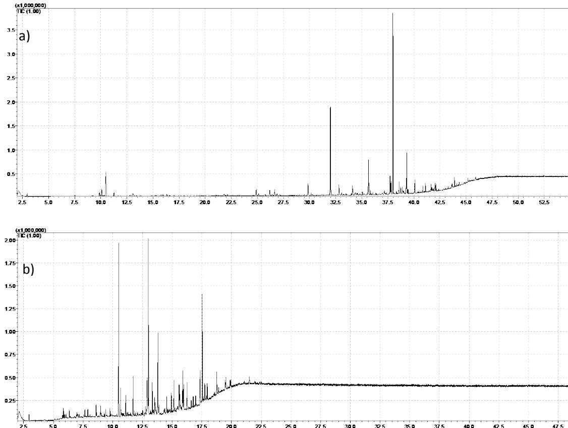
**Figure 4: Chromatograms of the upper layer material of fairing parts measured under a) VOC and b) FOG conditions**
